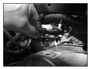
14. Remove the spark plug high tension leads.
