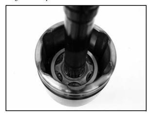
16. Use a soft-faced hammer to tap the joint onto the drive shaft until you reach the end of the splines and the joint locks in place.
