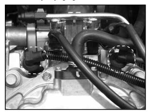
15. Disconnect the stator harness and crankshaft position sensor (CPS) harness or remove the (CPS) from the magneto cover.
