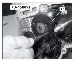
**NOTE:** Install the Cam Gear Tooth Alignment Tool (**PU-45497-2**) into the assembly hole counter clockwise from the timing mark as shown.
