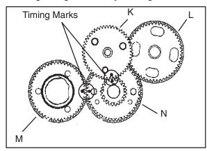
**NOTE:** It is recommended to replace all of the gears if any of the following gears are to be replaced:
