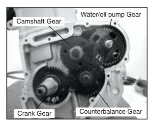
8. Use a white pen to accent the timing marks on the gears. This will ensure proper gear alignment and timing during reassembly of the gears.
