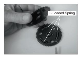
11. The cam gear assembly contains three loaded springs. To open the cam gear assembly:
